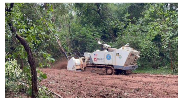
The Operation of Mini Minewolf Machine, which has been utilized together with other methods to destroy landmines
