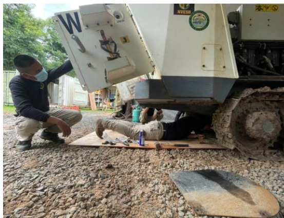
The Operation of Mini Minewolf Machine, which has been utilized together with other methods to destroy landmines
