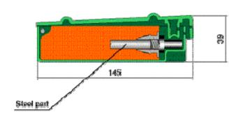
Length: 145 mm Width: 68 mm Height: 39 mm Mass: 400 g **Explosive charge:** 200 g TNT Plastic Body: Colour: Olive-drab Chemical Fuse type: Mode of activation: Pressure Sensitivity: 3 - 18 kps
