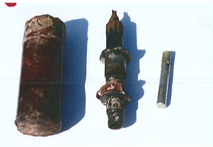
Picture 11: Main charge, ZZ-42 fuse and detonator from Stockmine found in the dunes.
