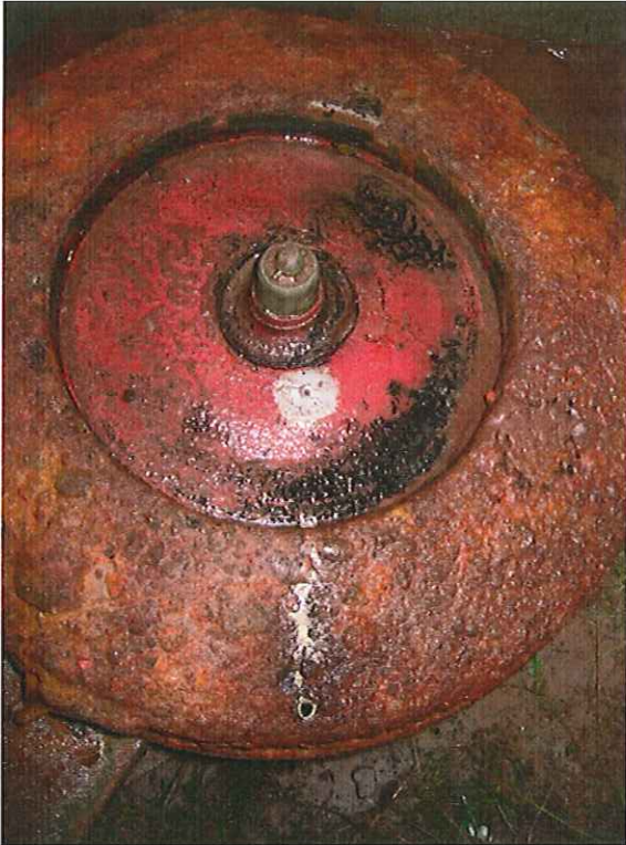
Picture 3: T-42 mine from Area 1. The mine has been opened with an abrasive water cutter, hence the water and sand on the fuse.
