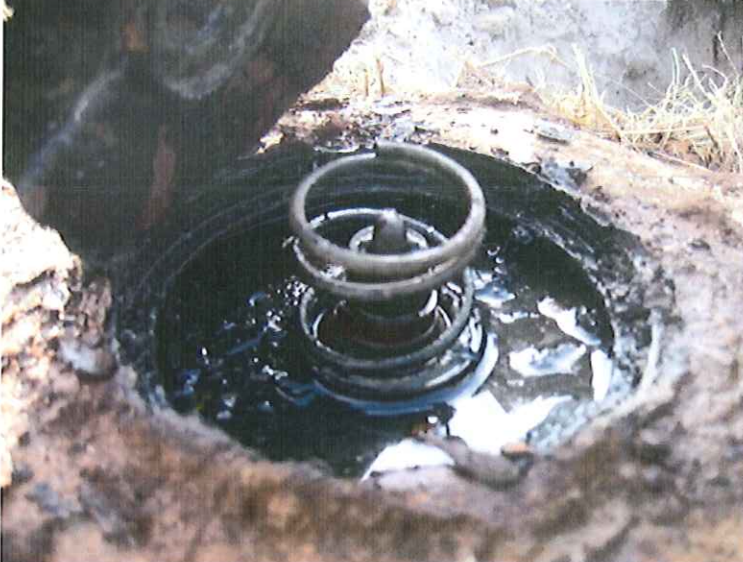
Picture 6: The inside of the T-42 found during the technical survey in Area 3 marshland. The fluid is oil from the attempt to loosen the fuse from the fuse well. When opened, the inside seemed unaffected by the wet environment in which the mine had been for 60 years.
