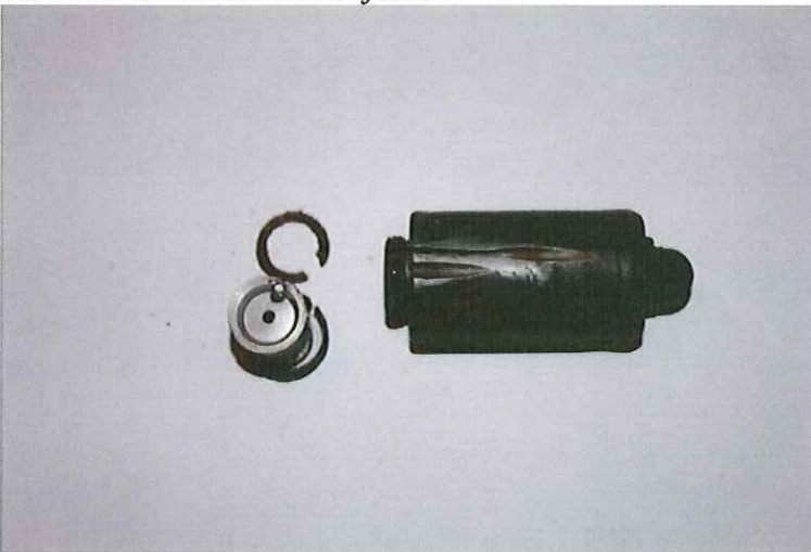
Picture 4: T-Mi.Zdr.42 fuse recovered from a T-42 mine in Area 1. The damages on the fuse body are made in the water cutting process.
