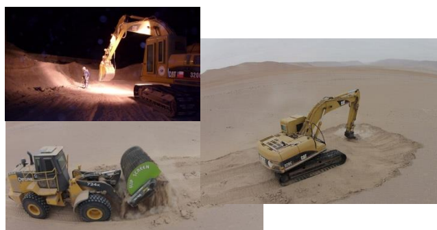
Mechanical clearance, Quebrada Escritos, Arica Sifting Excavator—Demining Loader
