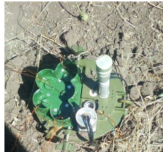
OZM-72 with a seismic target sensor
