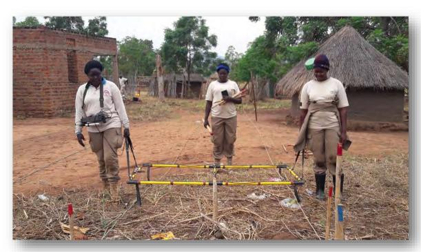
The clearance of cluster munitions is done using "large loop" detectors which can be calibrated to discriminate the size of signals and thereby allow for swift clearance as only the targets that generate a reading less than that of a cluster munition can be ignored.
